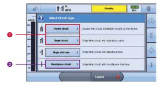
Mouthpiece ventilation can be set up with valve circuits ① or the mouthpiece circuit ② . The mouthpiece circuit is a simple, single circuit in which the mouthpiece can easily be replaced by a vented mask for night leak ventilation, without any need to change the circuit.
